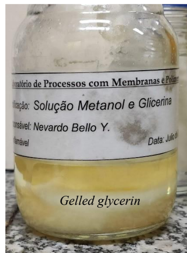
Figure 4.1. Obtained products. a) FAME-rich phase; b) Alcohol phase: Glycerin (white solid) + Methanol
